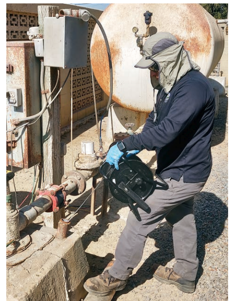
Conducting a well sounding to check water levels in the Basin.
