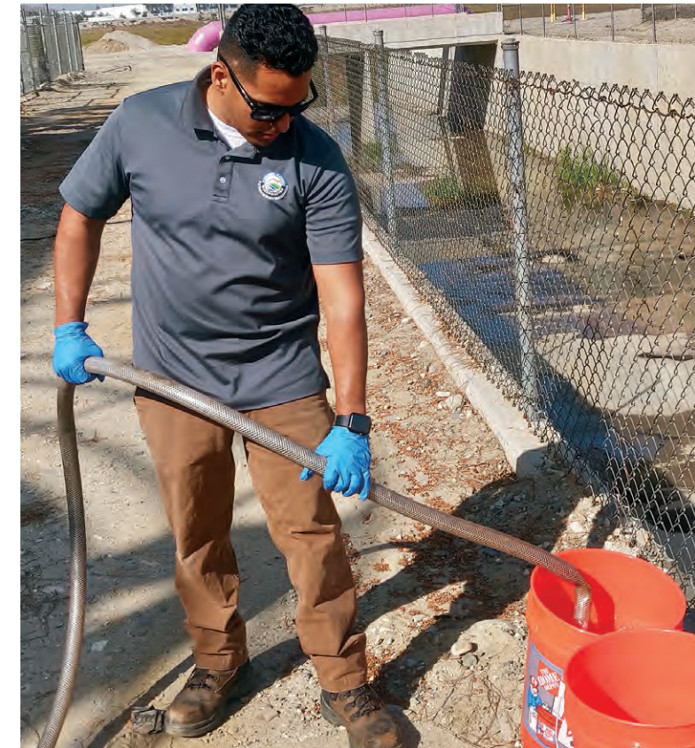
A Senior Field Operations Specialist purging a well for water quality sampling.
