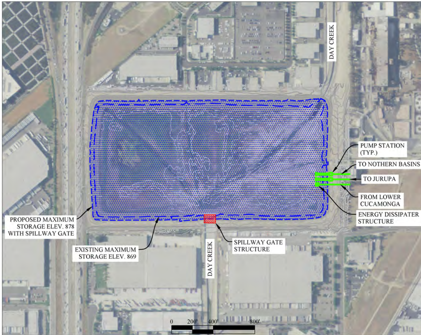
Figure 5-43 Wineville Basin Evaluated Alternative Schematic
