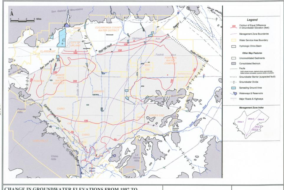
CHANGE IN GROUNDWATER ELEVATIONS FROM 1997 TO ULTIMATE CONDITIONS WITHOUT OBMP
