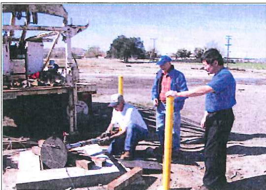
Watermaster operations staff preparing to pump a monitoring well to collect water quality samples
