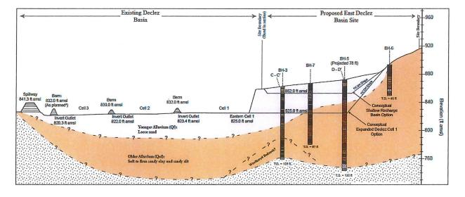
Profile of the proposed East Declez with bore hole testing locations
