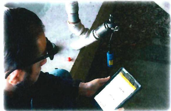
Setting a Transducer to Record Water Level Data
