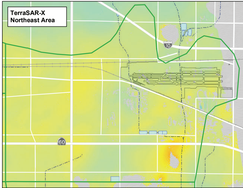
Figure 4 Sentinel-1A Versus TerraSAR-X Total Vertical Ground Motion Estimated across Northwest MZ-1 and Northeast Area June 2015 to May 2018 Chino Basin Watermaster Ground-Level Monitoring Committee
