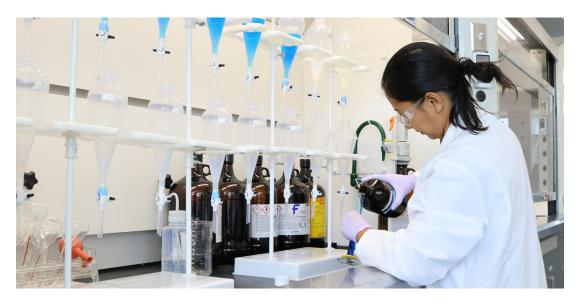
Quality Control Analyst performing Sufactants testing, a methane blue color reaction to detect the existence of anionic substances in water that may cause water corrosion or contamination.
