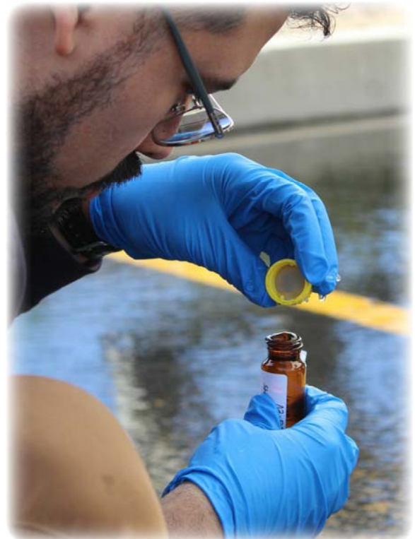
WM Staff Taking a Water Quality Sample to Test for VOCs
