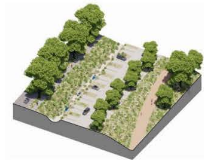
BIOSWALE NEAR PARKING
