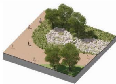
BIORETENTION/ DRY POND
