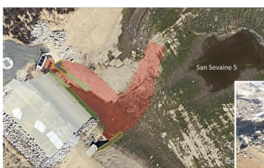
Grading basin floor near spillway, installation of riprap at storm drain inlet and riprap wave break near San Sevaine 5 outlet
