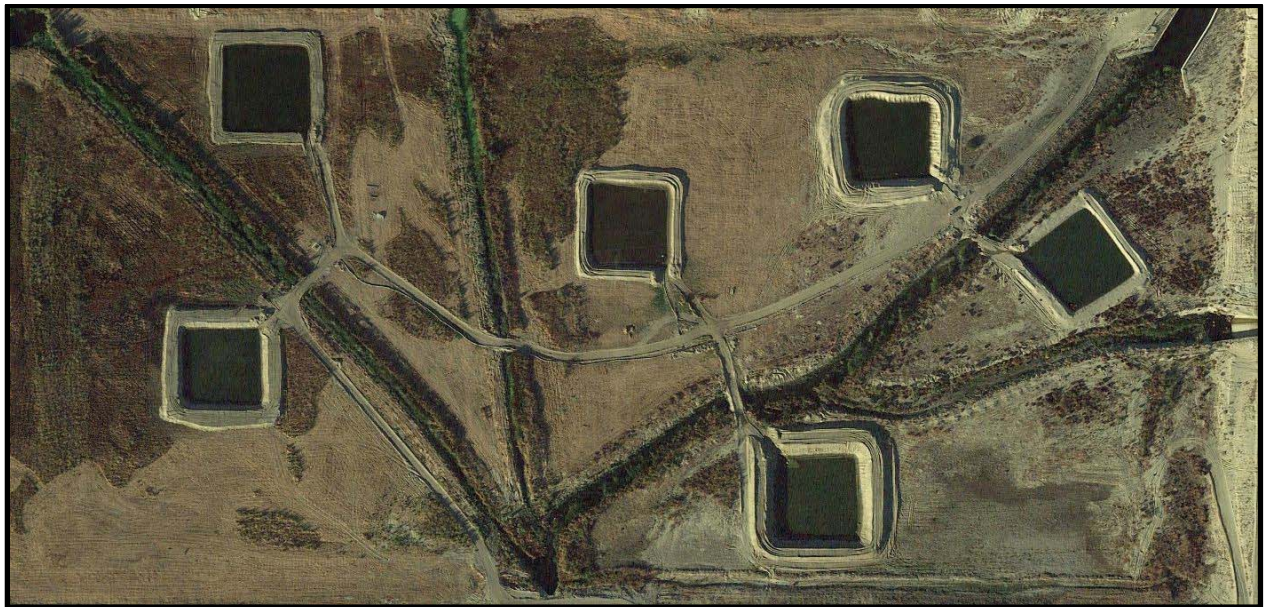
Figure 1- Image the of the temporary infiltration test cells constructed at Wineville
