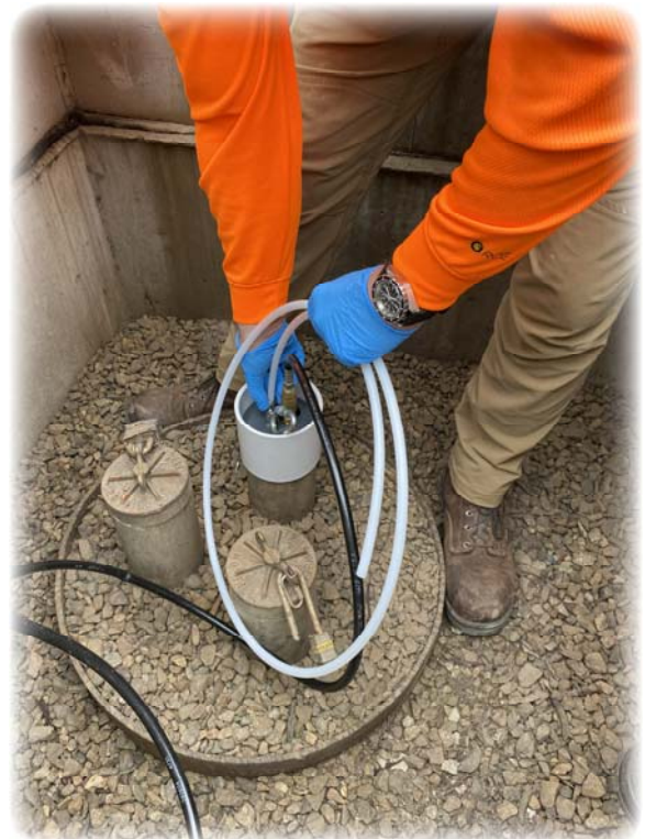
Preparing for Water Quality Sampling at a Monitoring Well
